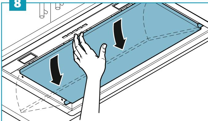
EN - Assembling standard active carbon filter: remove panel (8), re-move metal filters (9), assemble active carbon filters (10).
