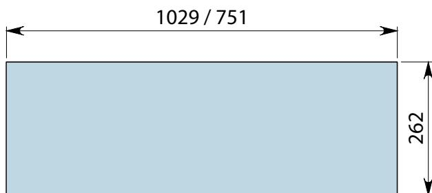
EN - Hole measurements for installation.
