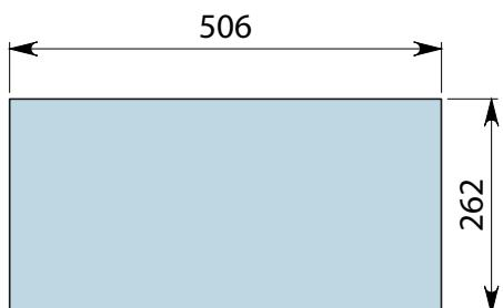
EN - Hole measurements for installation.
